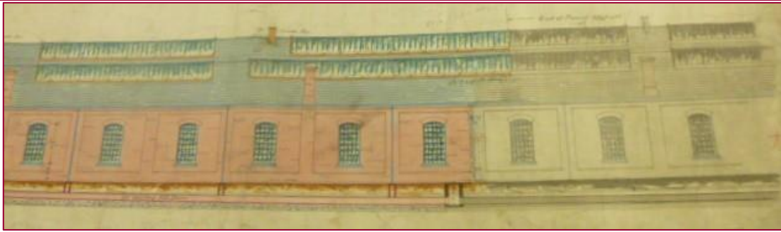
A drawing reproduced from the 1890 NER tender documents relating to the proposed extension to the existing S&DR shed. The western extension is coloured. Three turntables were to be incorporated inside the extended NER shed, replacing those built on the same site by the S&DR. (NATIONAL ARCHIVE Ref. 'RAIL 527/613')
