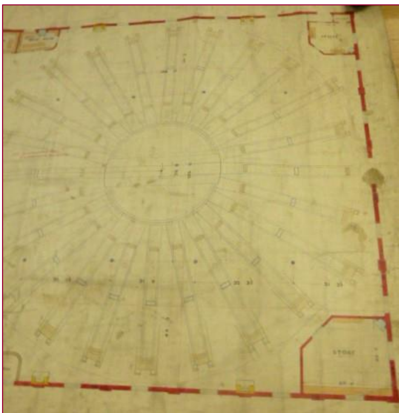
Another tender document plan from 1890 showing the existing turntable within the engine shed with the former store/ foreman's office in the top right corner.
