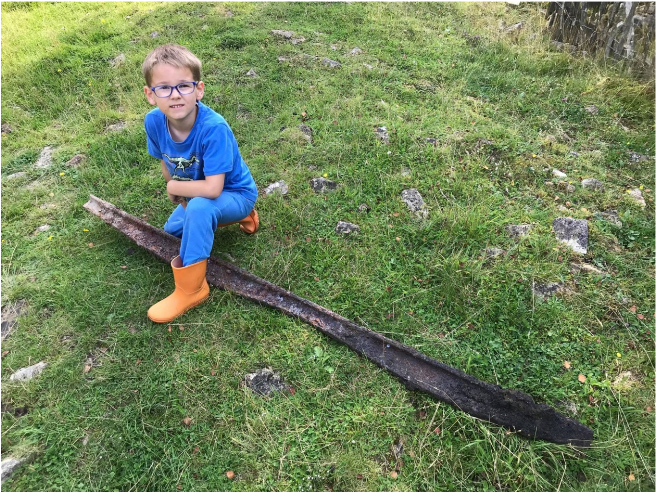
Seth Cooper with his amazing discovery of a fish belly rail on Cockfield Fell
