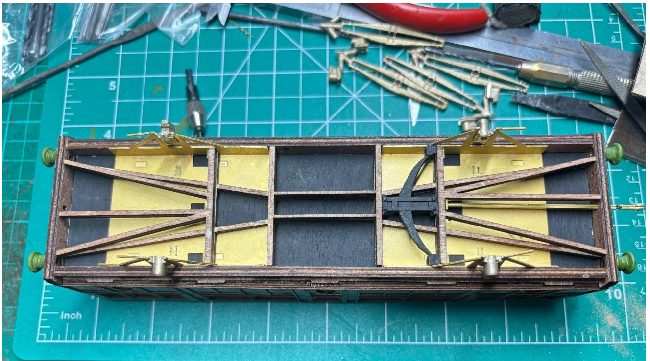
Smoking Carriage underframe construction
